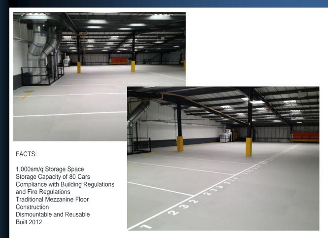
The whole project was completed from start to finish in just 6 week and on time and on budget. As a solution the project was 50% of the cost of a steel and concrete solution and obviously a great deal less than obtaining additional car storage off site, but the biggest benefit is the dynamic ability of being able to dismantle and reuse the Mezzanine either as a Car Storage Solution or a Standard Mezzanine Floor.
